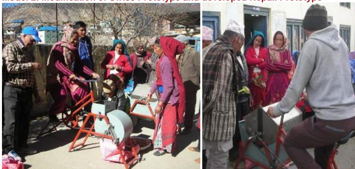
Picture: Performance test of walnut machine after first modification at Jumla, Dec 2017.
